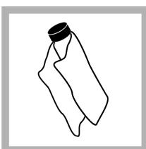
6. Use the oiling cloth to apply the oil equally to the surface of the vial. Remove most of the oil. Make sure that the vial is almost dry.
