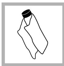
9. Use the oiling cloth to apply the oil equally to the surface of the vial. Remove most of the oil. Make sure that the vial is almost dry.
