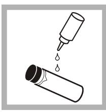
6. Apply a small bead of silicone oil from the top to the bottom of the sample cells.
