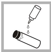
8. Apply a small drop of silicone oil from the top to the bottom of the vial.
