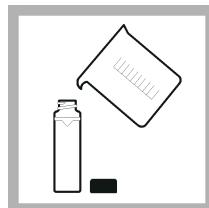
4. Rinse a clean, empty sample cell two times with the solution to be measured and drain to waste. Fill to the line (about 30 mL) with sample and immediately put the cap on the sample cell.
