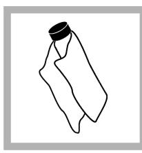
5. Clean the sample cells with a soft, lint-free cloth to remove water spots and fingerprints.
